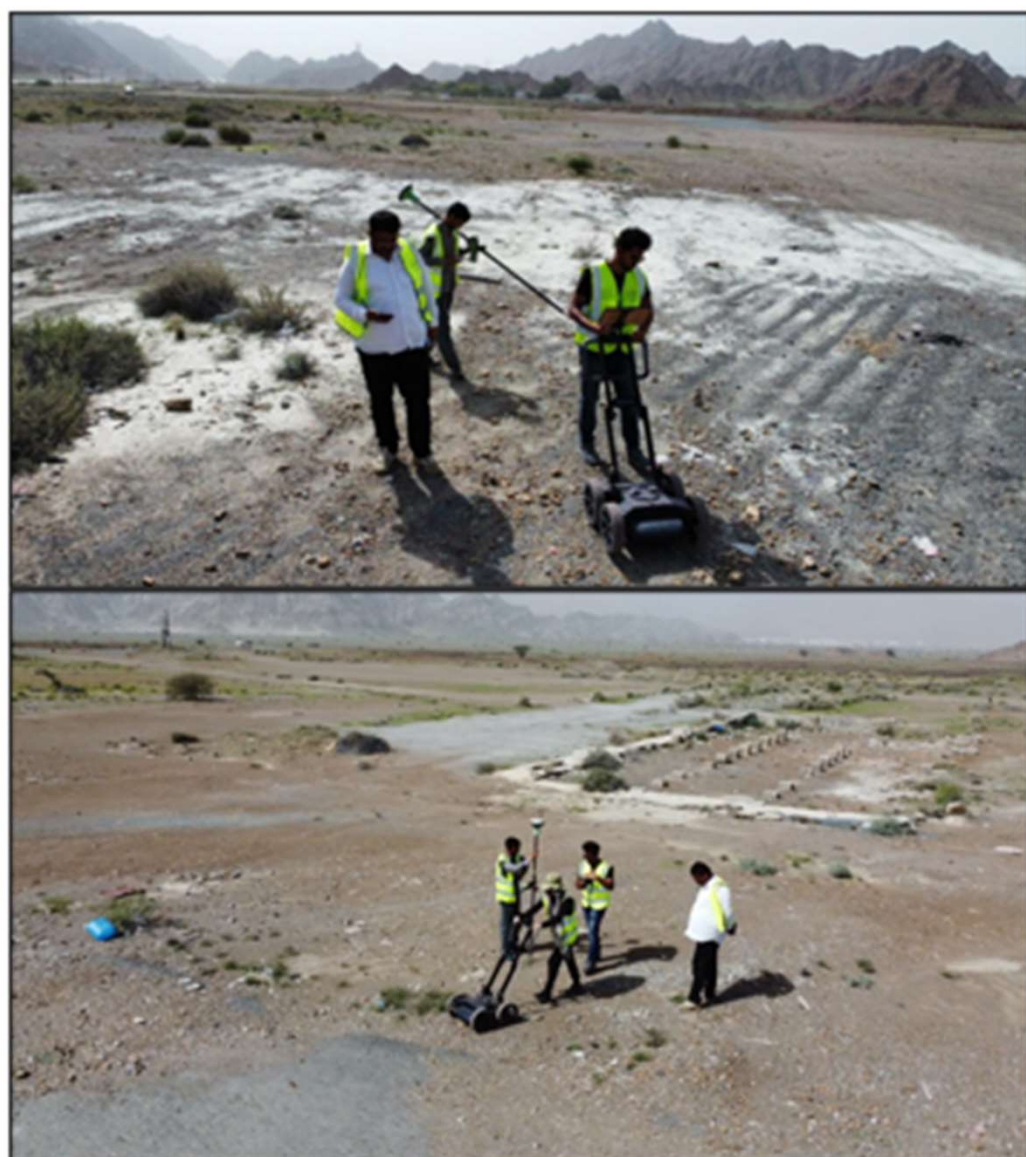
Figure 16 - GPR profiles acquisition with positioning equipment
